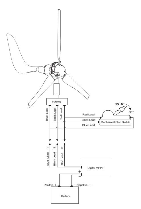
We strongly advise the activation of the mechanical stop switch during any maintenance of or around your Turbine. This will prevent the blades spinning and voltage to be transferred. Likewise during initial installation please activate the mechanical brake. The final step in installation of Turbine, controller, and battery should be release of this mechanical stop switch.
